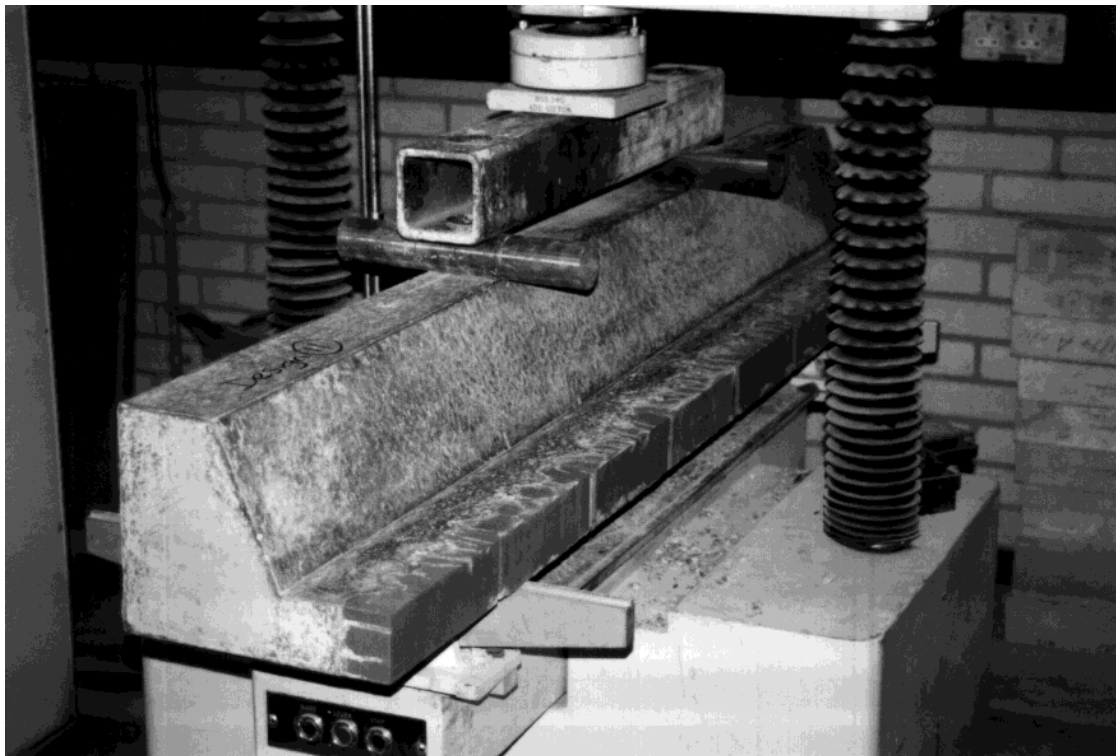
Plate 2: One of the lintels during testing
